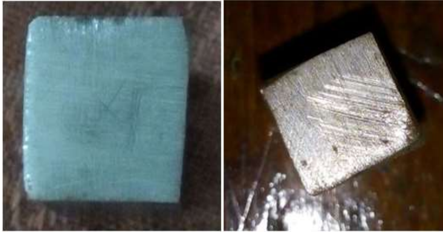
Figure 7 – Worn-out Surfaces of EN8 and Mild steel
